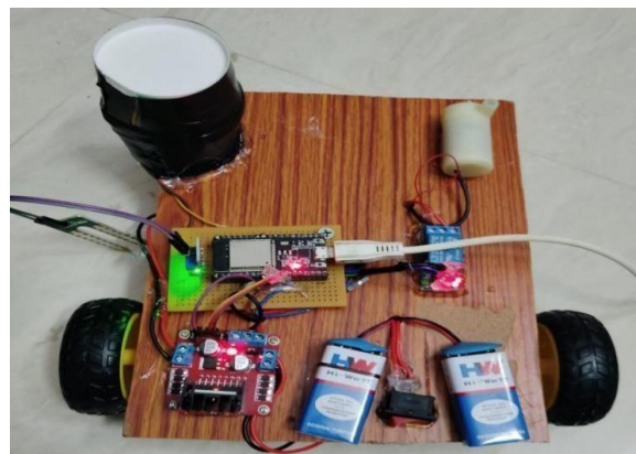
Figure 5 :Final Hardware Implementation of IoT-Based Multipurpose Agriculture Robote
